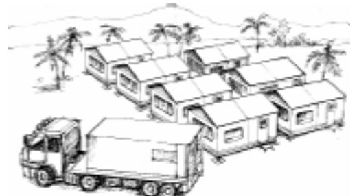
Seven 5m x 3m housing units supplied as 'flat pack' kits in one standard container
