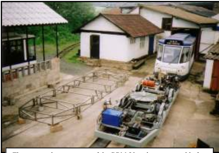
The principal components of the PPM 50 railcar, pictured before final assembly at Parry Associates' Cradley Heath workshops. The flywheel casing can be seen in the centre of the main chassis
