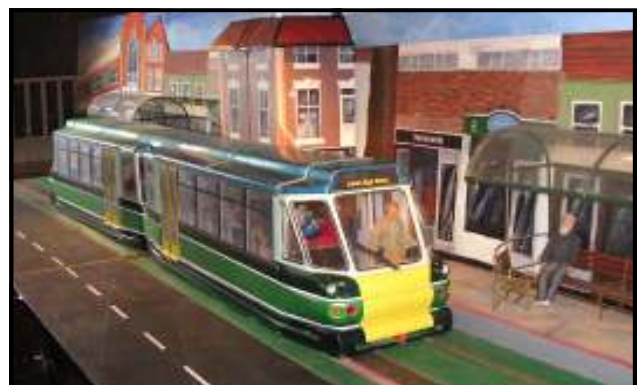
Visions of the future: Models showing a lightweight vehicle with corridor connections (left) and a twin-car set (below). Both illustrate the potential for low-floor trams suited to street running
